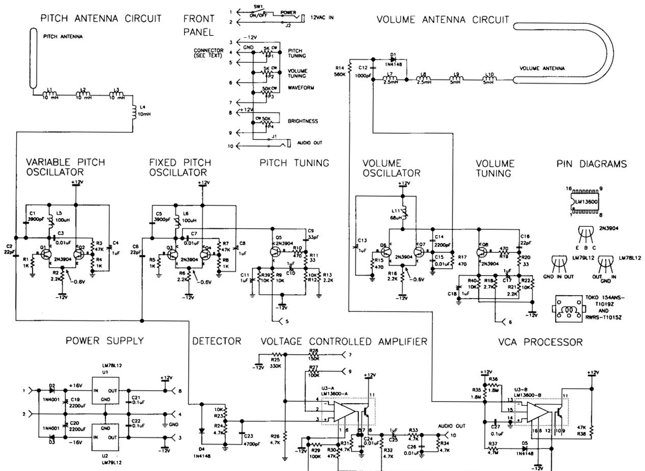
FIG. 2: The schematic for the EM theremin.
